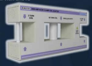
Designed for the calibration of both wound AC and magnetic field hall effect AC/DC clamp meters, the Transmille current coil offers several unique features.
