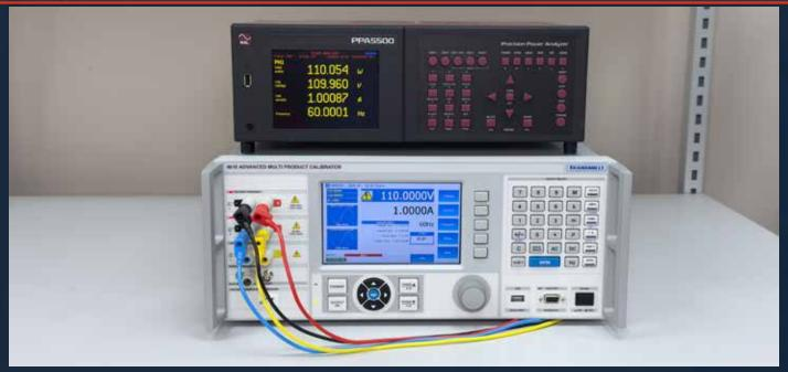
The PWRSINE option for the 4600A Series enables calibration of power meters, offering DC power output and AC power with variable phase between Voltage and Current outputs. Dynamic phase control enables calibration of both capacitive and inductive loads without additional error.
