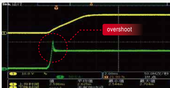
Diode load Conventional power test
