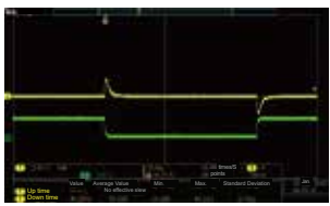
Standalone set IT6522C 80V, 120A, 3000W Voltage ratings: 10V Current ratings: 120A Load current: Level A=10A Level B=100A F=10 Hz
