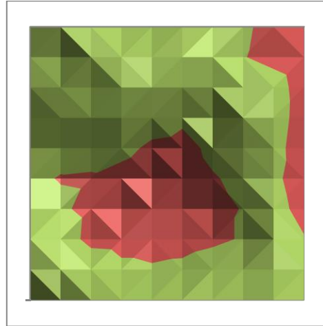
Typical non-uniformity map of an Abet Technologies model 11002 SunLite™ Solar Simulator, 50x50 mm; <5% standard
