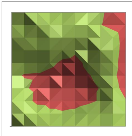
Typical non-uniformity map of an Abet Technologies model 11002 SunLite™ Solar Simulator, 50x50 mm; <5% standard
