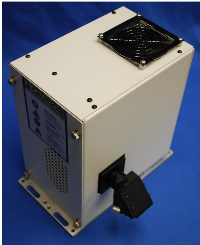
Abet Technologies Model LS 150 Light Source with a 20035S 45° mount with manual shutter, UV 280-400 nm
