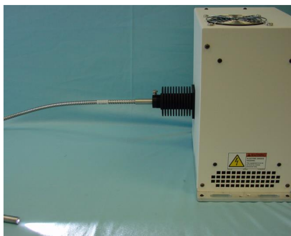
Abet Technologies Model LS 150 Light Source with a 20093 F/2 Fiber adapter and a fused silica fiber bundle
