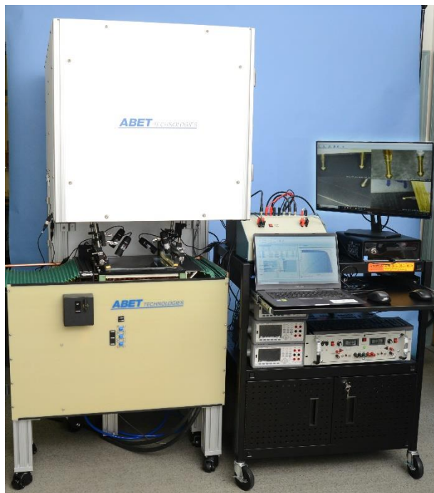
Model 15530SP 300x300 mm stage motorized chuck for CIGS mini-modules for automatic single cell and full mini-module IV metrology in use with a Sun 3000 Solar Simulator, a 15295 100V electronic load and four alignment microscopes. The simulator equipped with a filter wheel for Red and Blue and Attenuated measurements.
