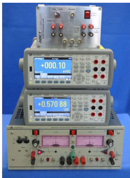
Elements of Abet 15295 Universal load, 10A capacity
